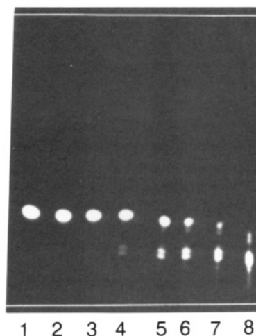
Figure 2. Autoradiography of the TLC analysis in \text{CHCl}_3/\text{MeOH}/\text{AcOH} (85/10/5) of the time course of photolysis of ^{125}\text{I} -HADM. Lane 1: ^{125}\text{I} -HADM (0.15 \mu\text{mol} ) in phosphate buffer I (1500 \mu\text{L} ). Lanes 2–8 represent photolysis for 10, 20, 40, 60, 120, 180, and 240 s, respectively.
